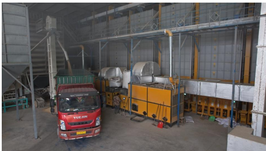
Figure 3 Grain drying line and postharvest facilities at Mashan Agricultural Service Center (Photoed by Xinfeng Ren)
