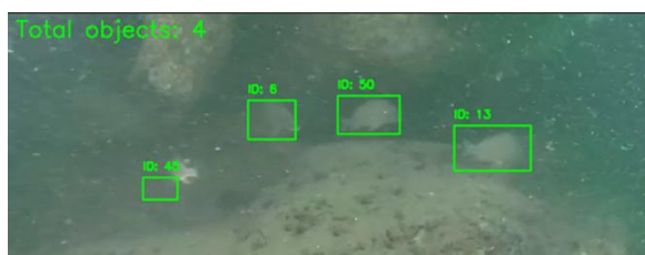
Figure 2 Fish counting results show the number of objects with bounding boxes in each frame (Adopted from Khiem et al., 2025)
